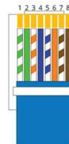
RJ45 Pinout T-568A
